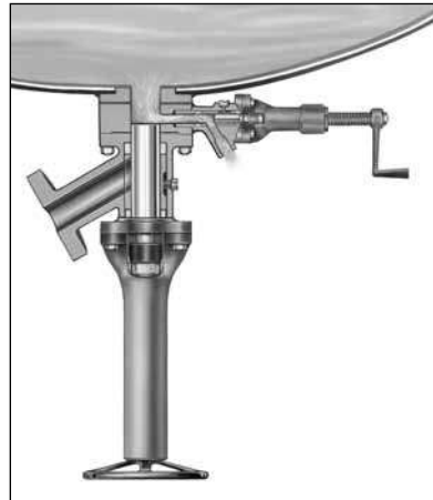
Fig. 2 - Drain Valve Open for Sample
